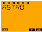
Press OK to confirm the ASTRO menu. Then press button ► four times and press OK to confirm.
