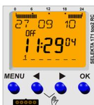
Either confirm with OK or modify the changeover rule for the automatic summer/winter time switchover with the arrow buttons and then confirm by pressing OK.
