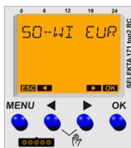
Either confirm with OK or modify the minutes (flashing) with the arrow buttons and then confirm by pressing OK.
