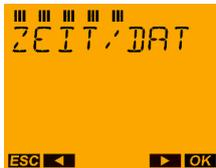
Press the OK button, then the ► button six times.
