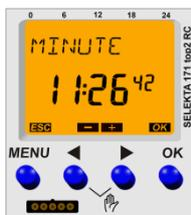
Either confirm with OK or modify the hours (flashing) with the arrow buttons and then confirm by pressing OK.
